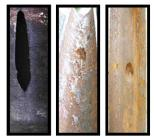
Flaws Shown Above From Left To Right Rod Wear Split, Internal Pitting, Pitting With Hole
