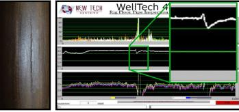
Left: Longitudinal Split In Tubing From Rod Wear Right: Split Detected With WellTech Software
